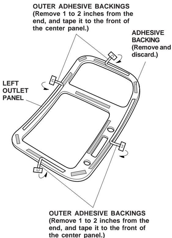
9. Position the left outlet panel on the outlet in the position noted in step 7. While holding pressure on the outlet panel, slowly and carefully remove the adhesive backings from the outlet panel. Hold the shift panel firmly against the existing shift panel with the palm of your hand for 30 seconds.
