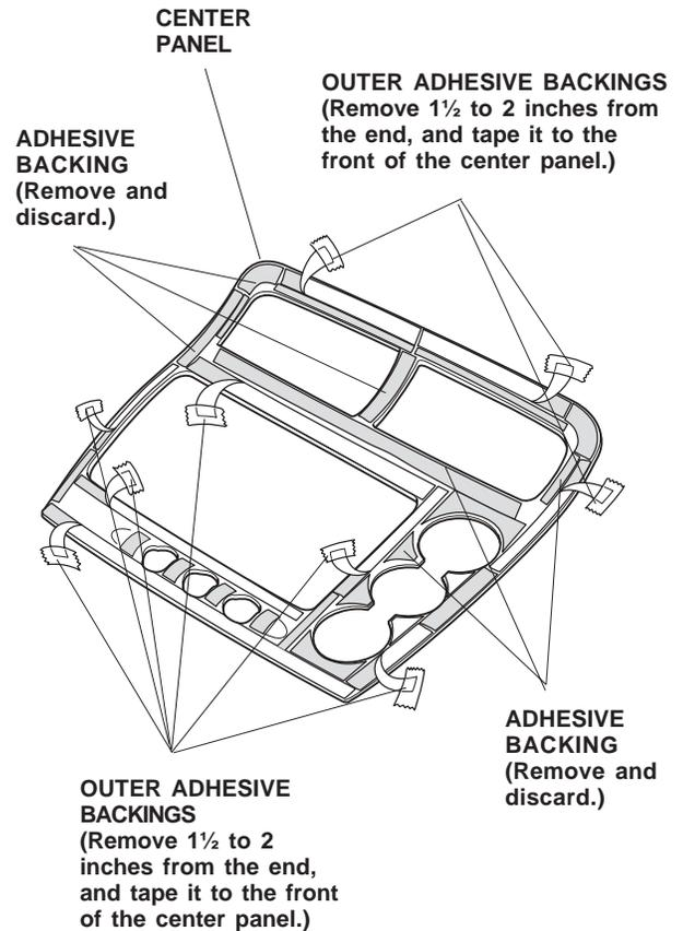
3. Angle the center air outlet louvers down. Position the center panel on the existing center panel in the position noted in step 1. While holding pressure on the center panel, slowly and carefully remove the adhesive backings from the center panel. Hold the center panel firmly against the existing center panel with the palm of your hand for 30 seconds, particularly at the edges.
