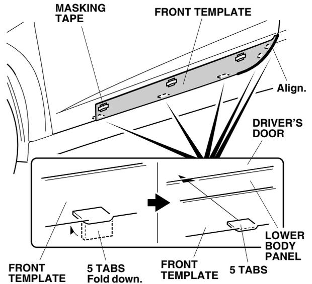
4. Align and attach the front template to the driver's door with masking tape.
