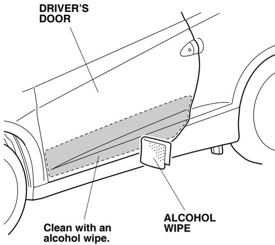
2. Using one alcohol wipe, thoroughly clean the driver's body panel where the left rear body side molding will attach.
