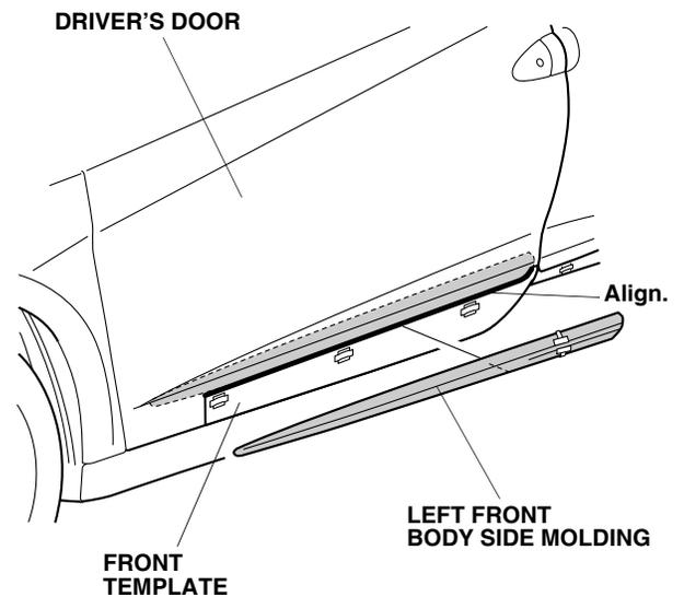
9. Peel back approximately 1½ to 2 inches of adhesive backing from each adhesive tape, and tape the ends to the front surface of the body side molding. Remove the end pieces of the adhesive backing.
