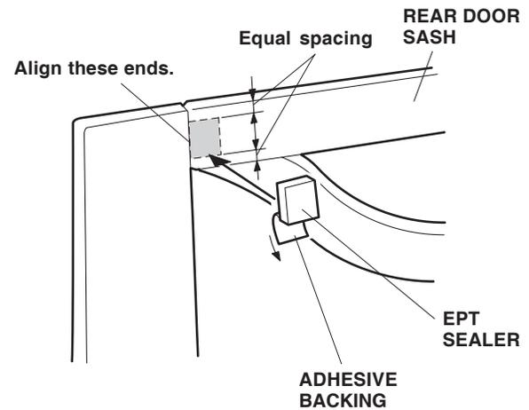
13. Attach a strip of masking tape to the end of the adhesive backing at the rear of the door visor, and remove 2 to 3 inches from the end. Fold back the end and tape the end to the back of the door visor.
