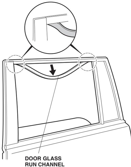
11. Using isopropyl alcohol on a shop towel, clean the shaded area of the door sash.
