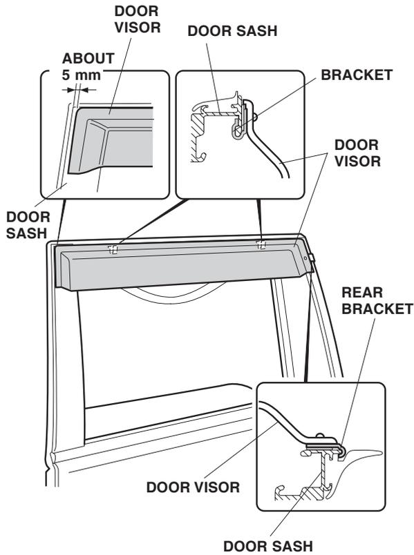
16. Adjust the location of the door visor so that the clearance between the door visor and door sash is about 5 mm at the top.
