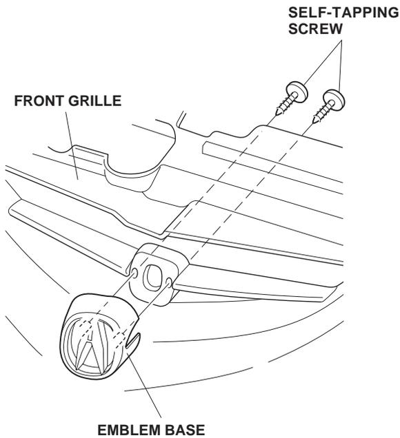
3. Using diagonal cutters, cut the locating tabs from the existing front "A" emblem. Push the locating tabs to remove the emblem from the emblem base.
