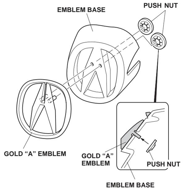
6. Reinstall the emblem base and front bumper. Check that all clips are installed securely without play or lifting.
