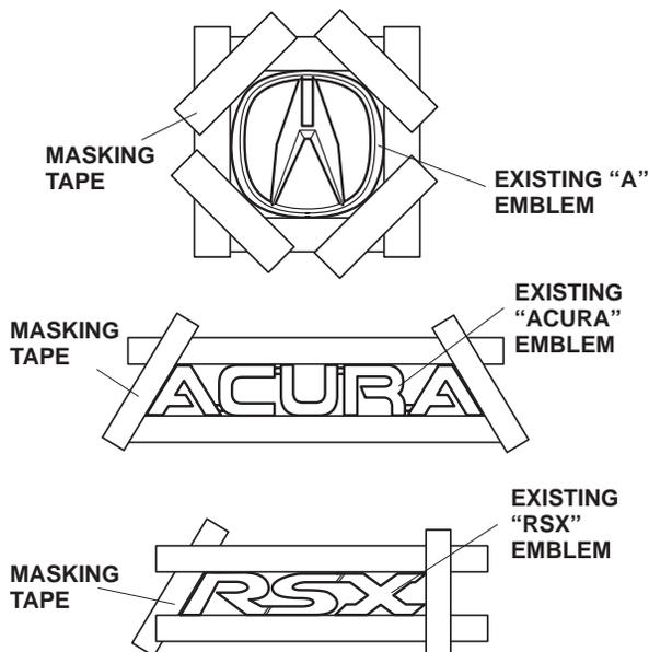
8. Using string, remove the emblems from the body by moving the string in the directions shown. Note the locating tabs of the emblems when moving the string.
