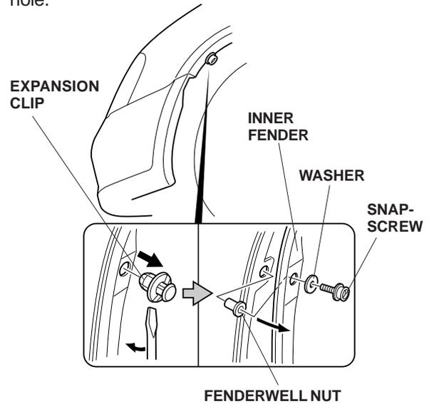
6. Pull the inner fender away, and press one fenderwell nut (supplied) into the hole in the fender flange.
