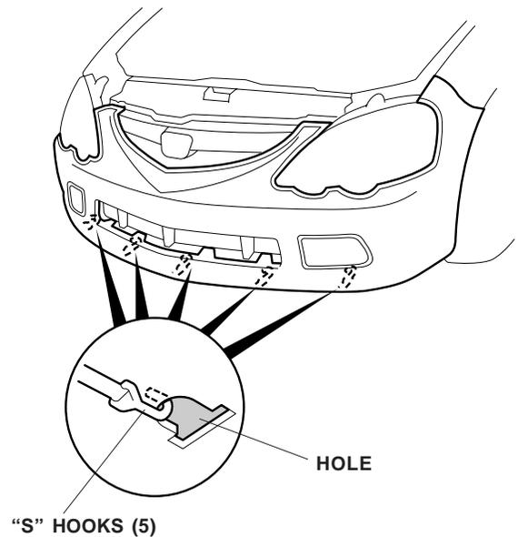
16. Route the two belts through the holes in the front grille, and attach them to the inner "S" hooks.
