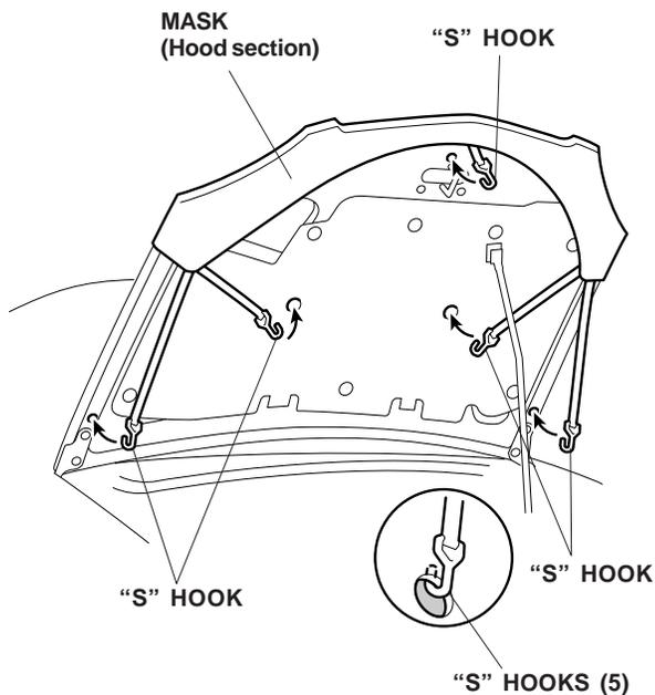
3. Secure the mask by hooking the four "S" hooks to the holes in the back of the hood.
